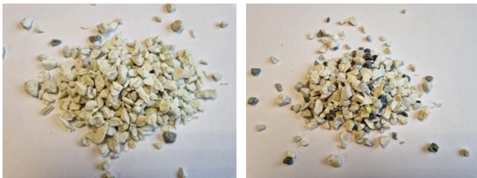
Regrinded plastic residues done by OMAPLAST (Left: PP GF; Right: PP TD + Talc + CaCO 3 )
