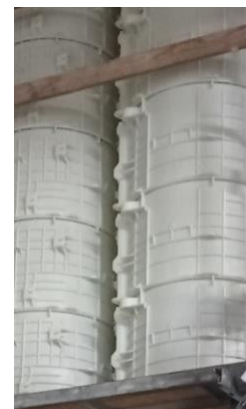
PP (GF) (Glass fibers 35 % - 50%) and final parts from production (uncolored examples)
