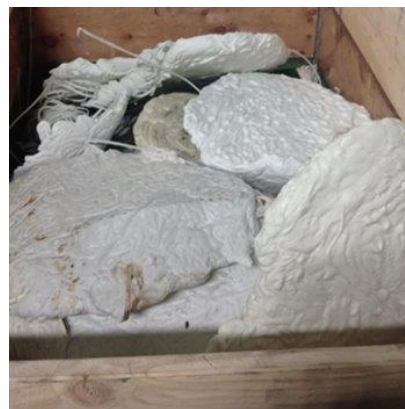
PP (GF) (Glass fibers 35 % - 50%) and final parts from production (uncolored examples)
