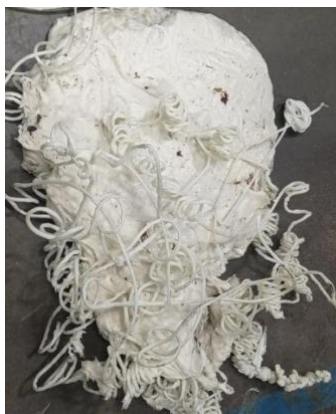
PP (GF) (Glass fibers 35 % - 50%) and final parts from production (uncolored examples)
