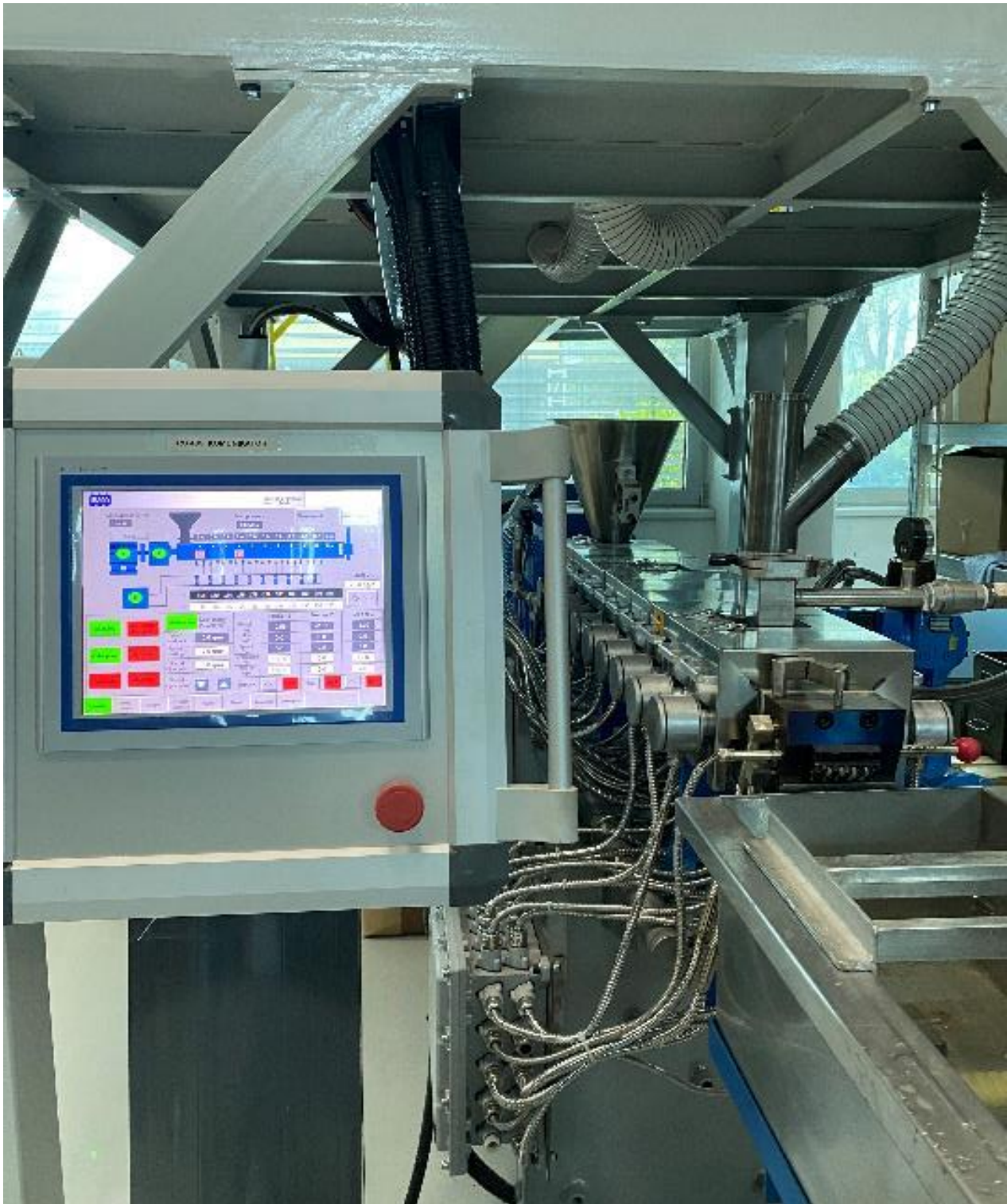
Figure 7: USEON Lab30 Compounder - Output: ~50 kg/h (depends on formula and operation conditions)
